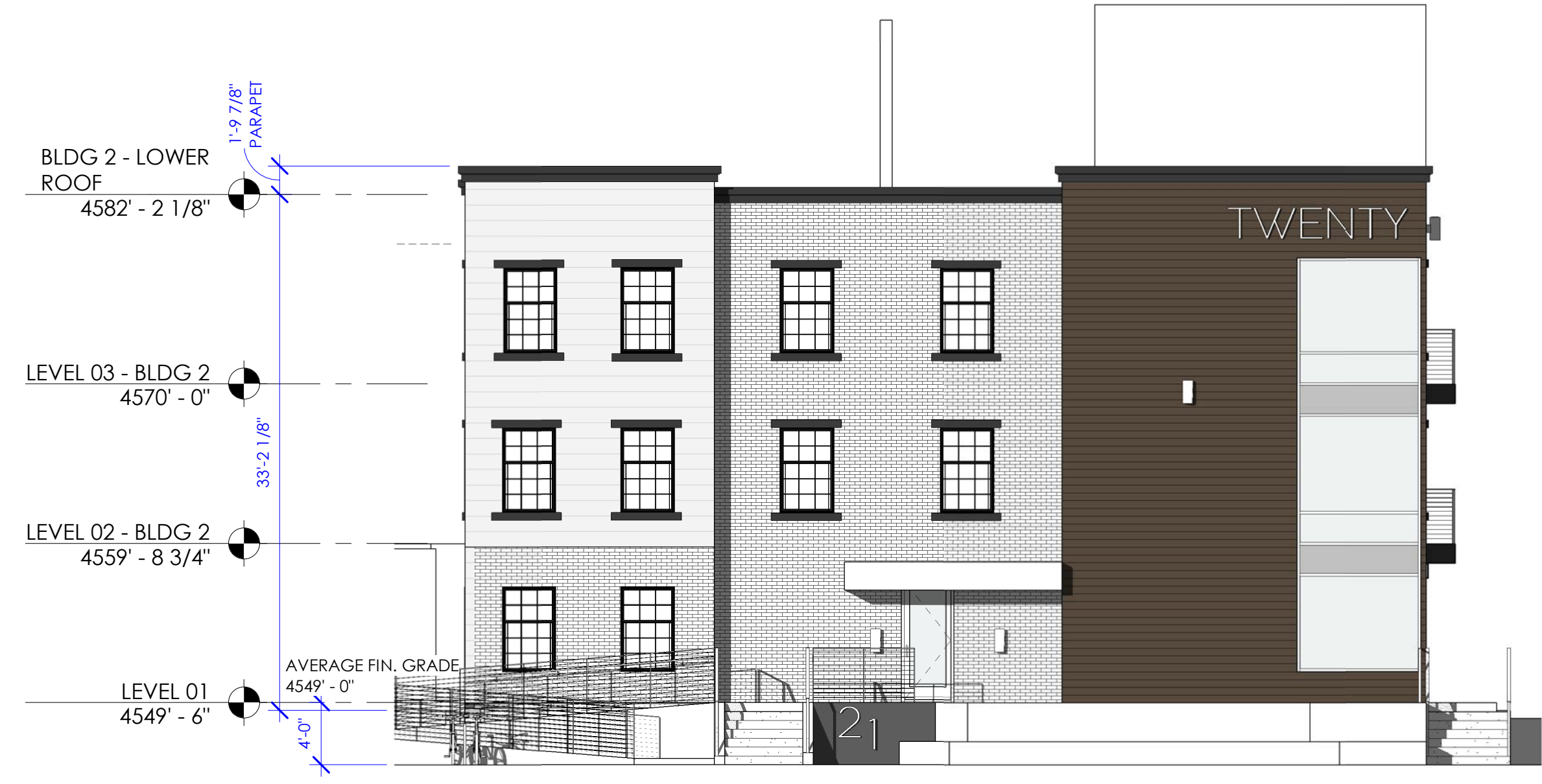
3 A206 BUILDING 2 - WEST ELEVATION 1/8" = 1'-0"
